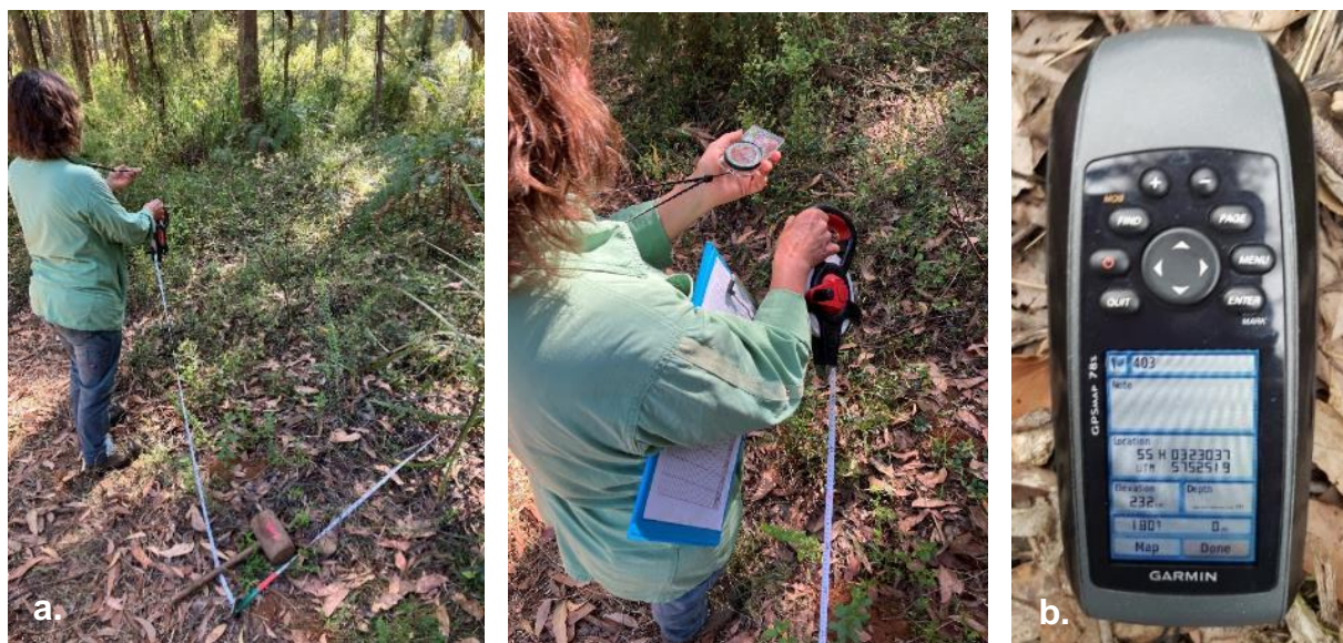
Figure 12. (a) Setting up a plot using a compass to determine direction of 20 m tape measure; (b) recording latitude and longitude of plot corner with a GPS.
